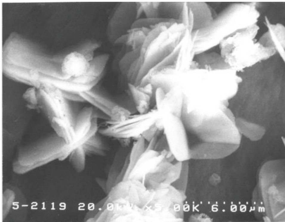
Figure 4. SEM-EDS photomicrograph of a uranium-rich grain on Apatite II from one of the columns. The plate-like structure is typical of the autunite mineral group and spectra indicate autunite (from MCLInc.).
