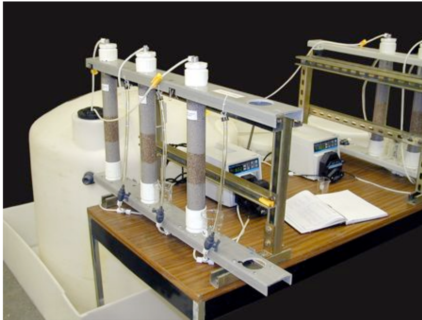
Figure 3. Column Studies for Apatite II Permeable Reactive Barrier at Oak Ridge Y-12 site. The Y-12 groundwater influent is contaminated with ppm levels of uranium (from MCLInc., and MSE, Inc.).
